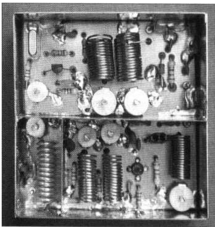
If you keep all values of the coils and capacitors as suggested then you can preset the following settings of the variable-capacitors before you start tuning.
