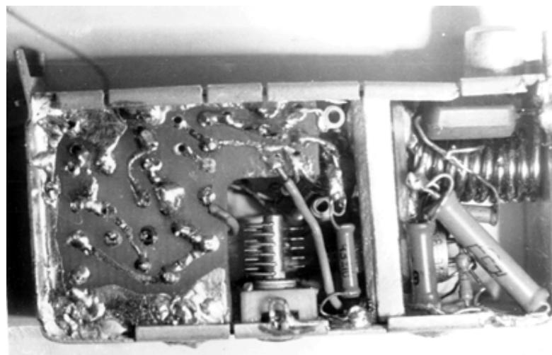
QRP CW Transceiver. View on the PC Board
