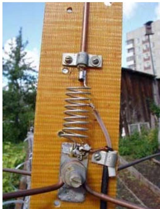
Of course, you can adjust the antenna with the help of only SWR – meter or VHF - bridge. There are 8 such home - made Bottle Antennas at Novgorod. All antennas work very well. They provide good communication as inside city as from city to a country for a distance more of 100 kilometers.
